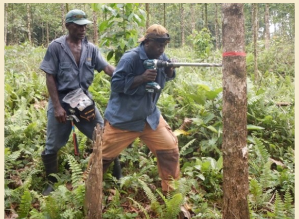
Mr. Steve Koloa assists Mr. Peter Mailagi to extract an increment core of a young teak tree in the Solomon Islands.
