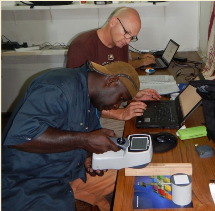
Mr. Peter Mailagi uses a color spectrophotometer to measure the colour of a teak sample at Munda Station laboratory.
