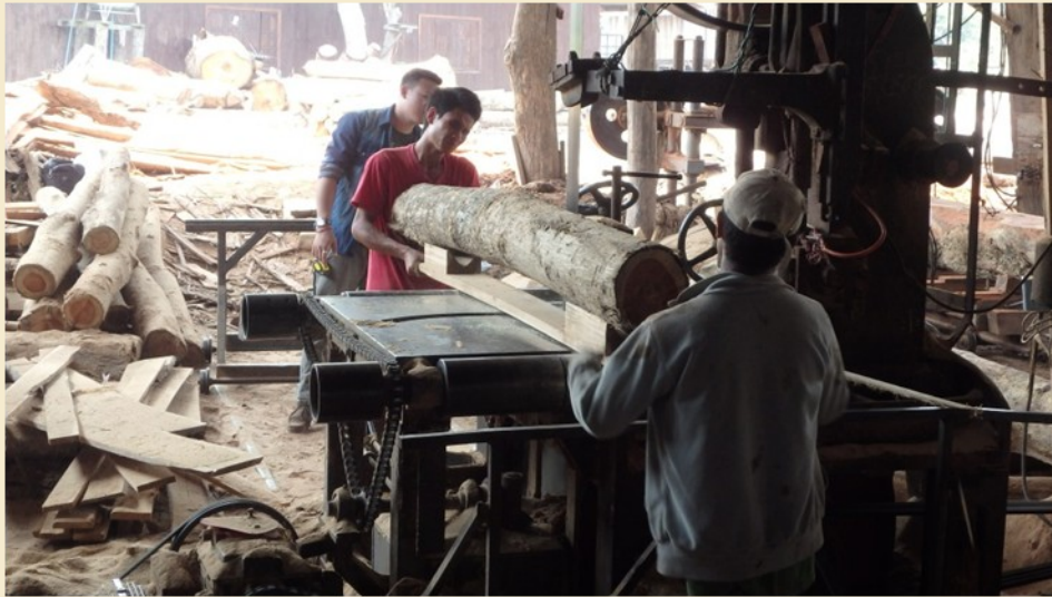
← Lao sawmillers using the DAF sawing jig to improve sawn accuracy and operator safety during teak sawmilling.
