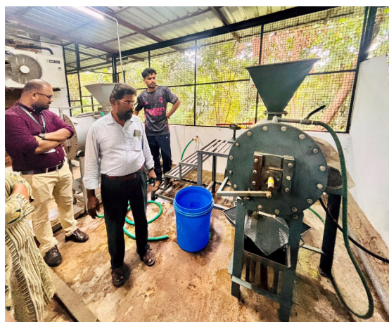
Dr. P. K. C. Pillai demonstrating the operation of a seed pre-treatment machine for scarification.
