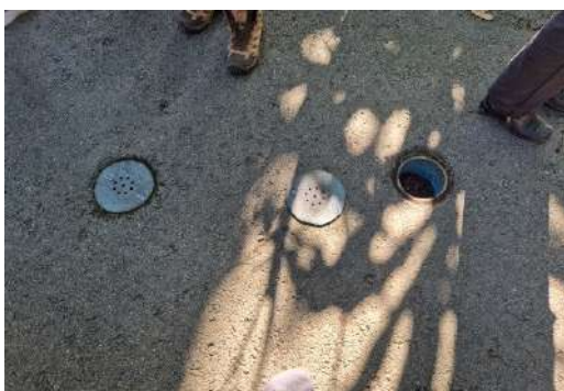
Soil compaction study methods digging holes and perforated PVC pipes in road pavement
